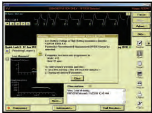
Example 1 – Programmer Software Detects Measurement Lock-up ERI
